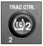
To enter this mode, press the TC2 button located on the instrument panel to the right of the steering wheel. If you restart your engine, the system reverts to the TCS mode.
